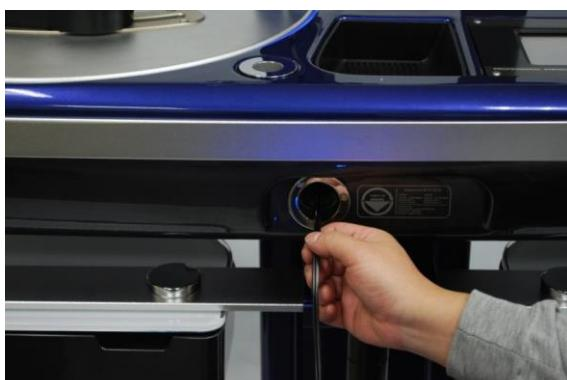
After using the Ironer, please put the cap back on the Ironer. Pull the wire softly, and the wire will pull back the stringing machine.
