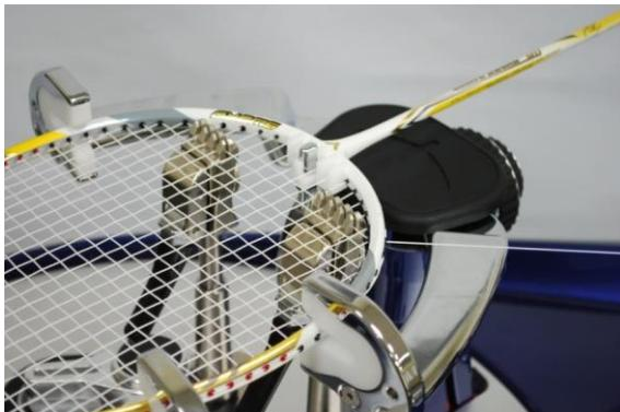
After finished the cross stringing, press the KNOT key will increase 10% of tension for knotting.
