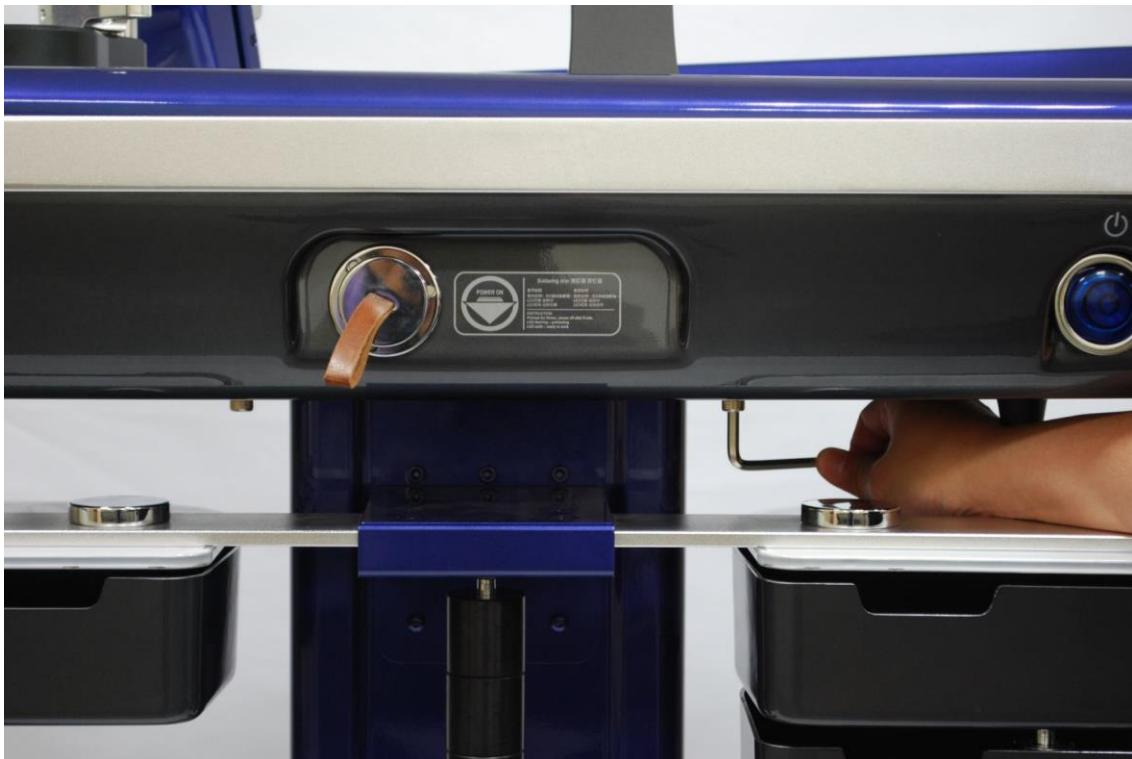
Fix the tension head on the machine base by using 6mm allen wrench to tighten the 4 screws (SOM8x25).
