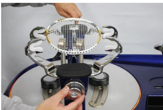
Then loosen the small knobs to open the tip/throat pins.
