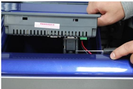
Lift up the touch screen and remove the signal terminal.
