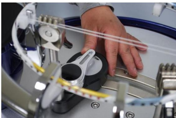
Move the Base locking lever clockwise to lock the clamp base.
