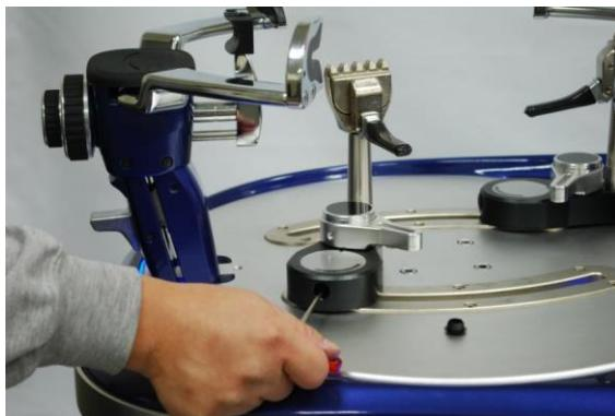
When the clamp base locking lever had been well locked but still feel some slight movement on the base. Move the base to the end of the rail and use a 3mm T-wrench to fine tune the screw as shown.
