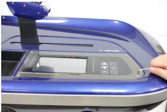
Use 2.5mm allen wrench to loose the 4 screws.
