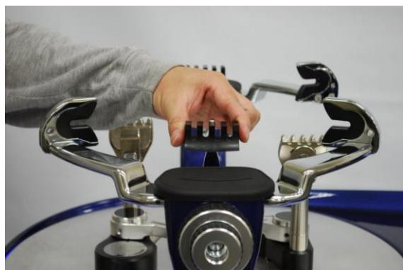
Insert the proper frame pad on the main pin.
