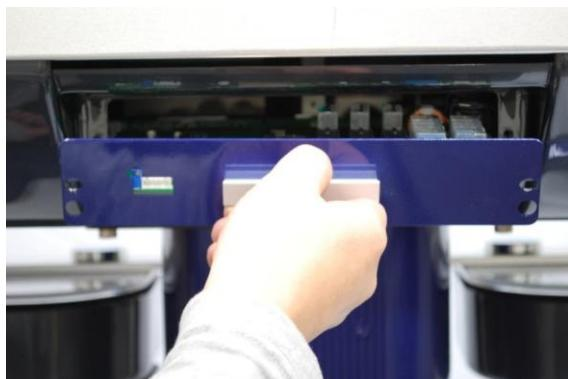
Pull out the PC board to replaced it.
