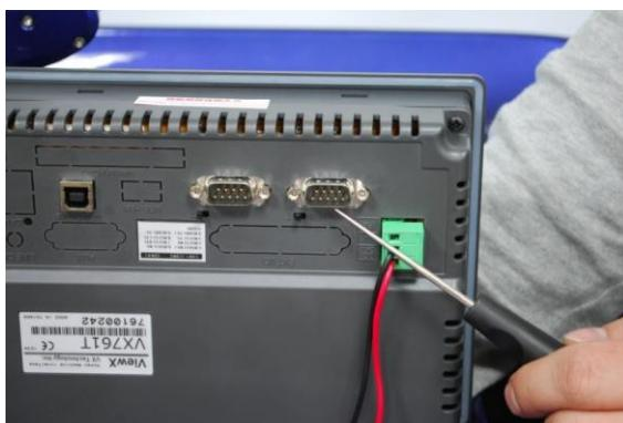
\* Please note the signal wire of touch screen should connect to the **C OM 1**.
