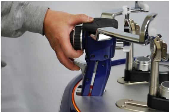
Lift the fix handle and pull out the post to the tennis mode position. The linear string gripper will switch to the tennis mode automatically.
