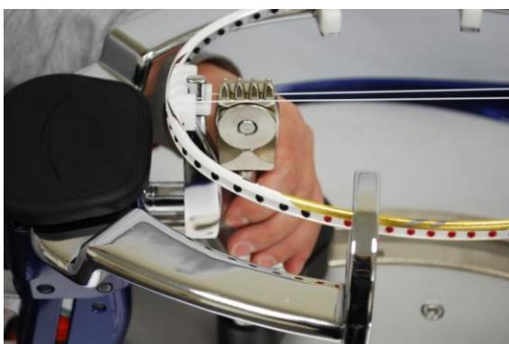
Apply one clamp to catch one of tensioned strings
