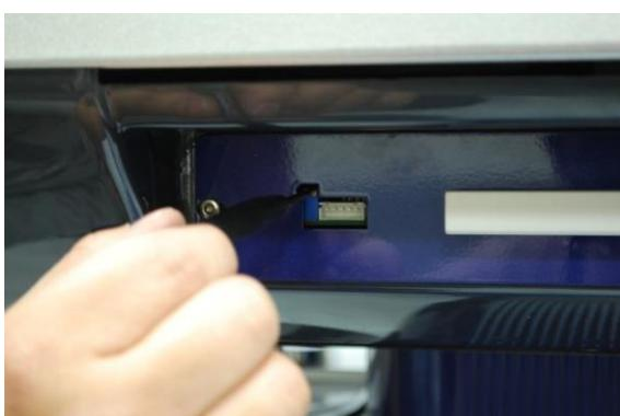
The tension adjusting should operate under the non-pulling condition.
