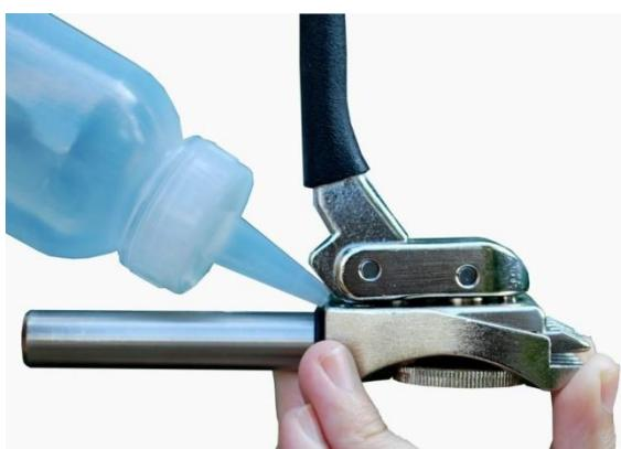
The contact surface of the string clamp handles receive a lot of compression while locking and unlocking clamp; therefore it is recommended to use Teflon based oil to keep this part well lubricated.
