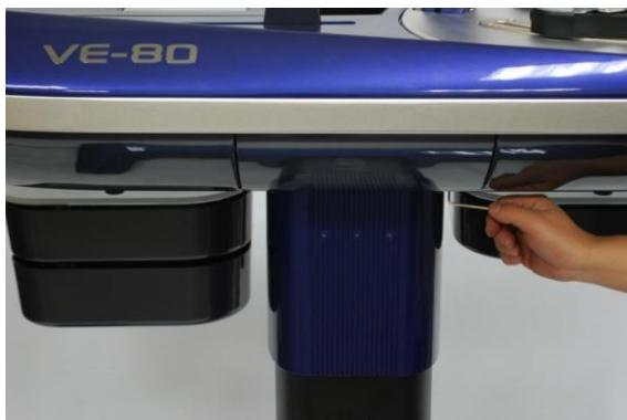
Using a 2.5mm L-shape allen wrench to loosen the 2 screws of the back panel and remove the panel will find the fine adjustment knob of tension adjusting.
