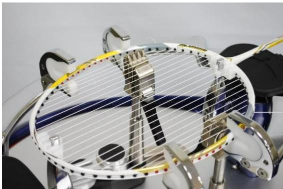
Repeat the same way pulling the string equally one by one until finish the last 2 main strings, pull the last one string first and then back to pull the last 2nd string ( Victor stringing way ).
