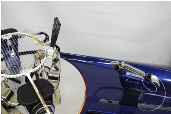
Apply a starting clamp to fix this string, not knotting yet.
