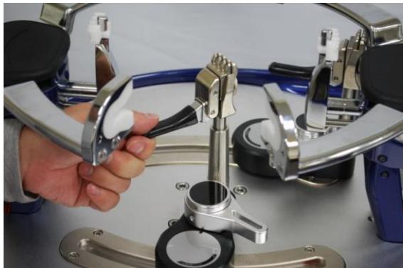
Open the clamp handle and let it fall down can release the clam base at the same time.
