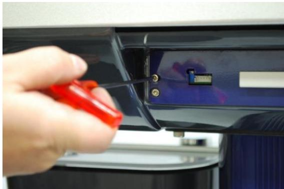
Use 3MM allen wrench to loose the 2 fix screws
