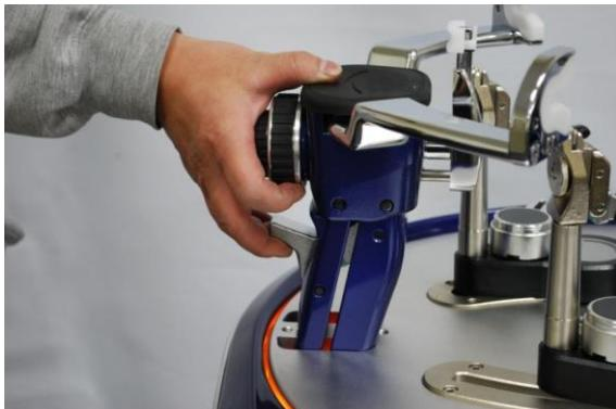
Lift the fix handle and push the post toward inside to the badminton mode position. The linear string gripper will switch to the badminton mode automatically.
