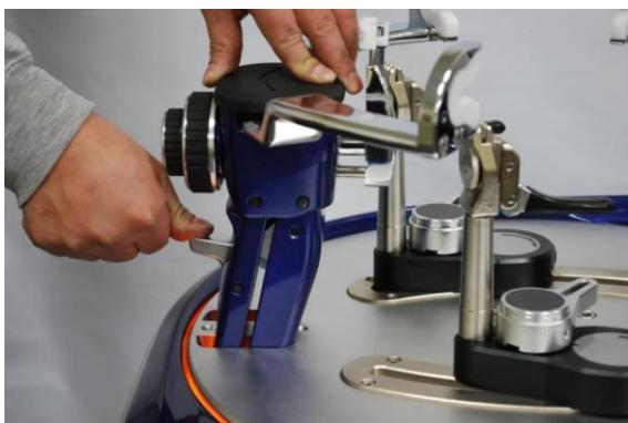
Push down the fix handle to fix the post.
